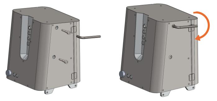
• Warning: If the cylinders dont rotate after turning the machine on, immediately disconnect the machine from the electrical socket and adjust the pressure of cylinders again.
